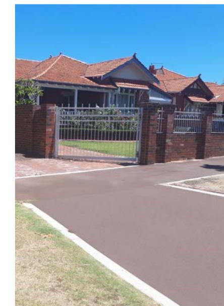
Image 9. Image shows red asphalt footpath priority over residential driveway. Source: UDLA.
