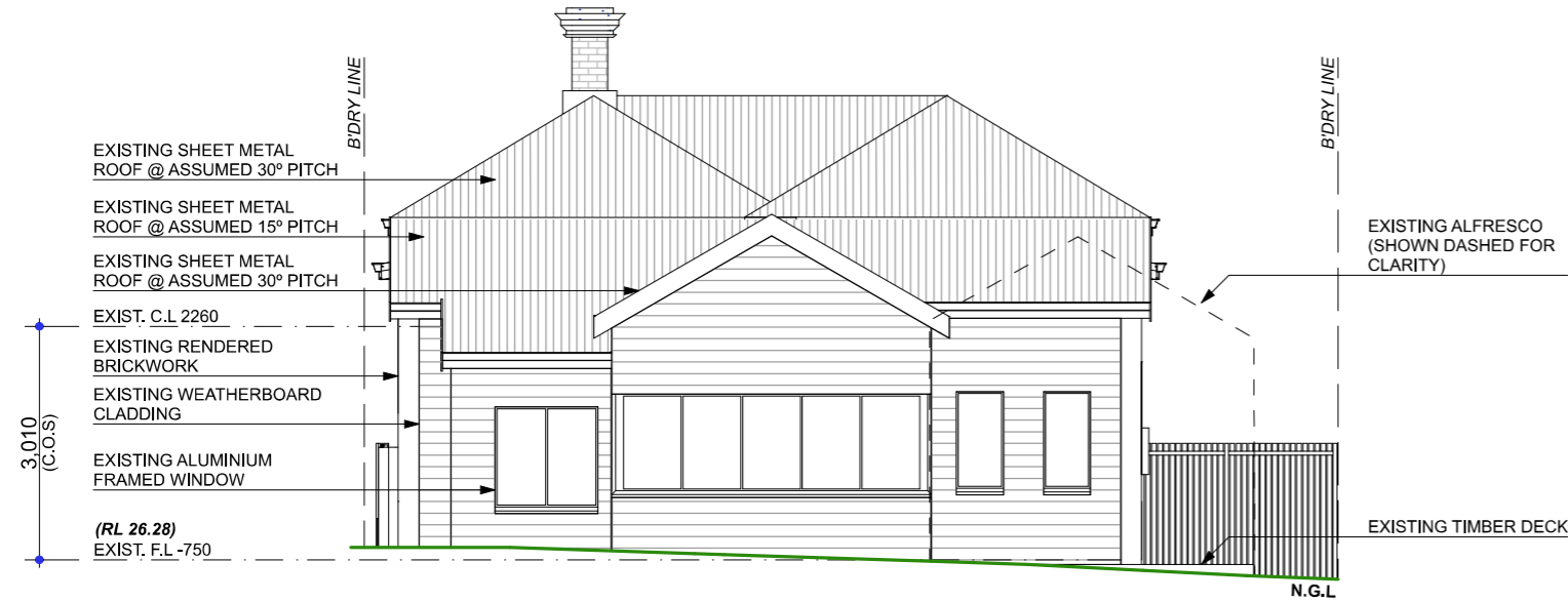
E03 A02 EXISTING ELEVATION 03 - EAST 1:100
