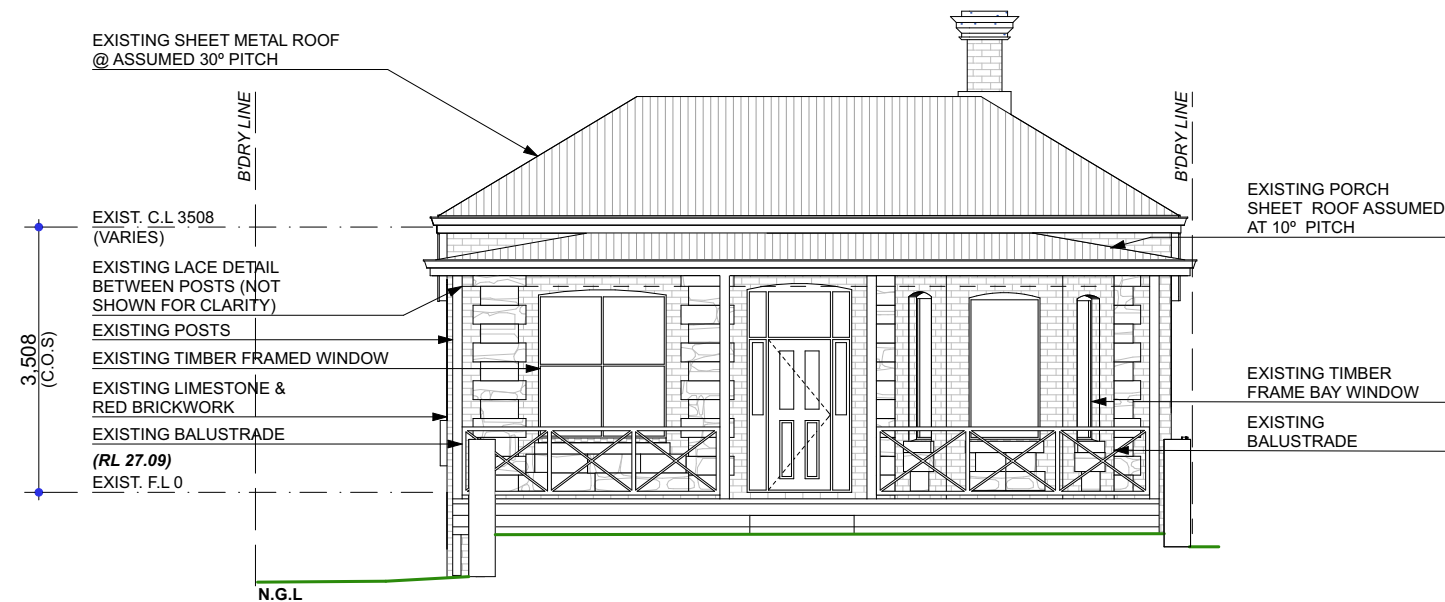
E01 A02 EXISTING ELEVATION 01 - WEST 1:100
