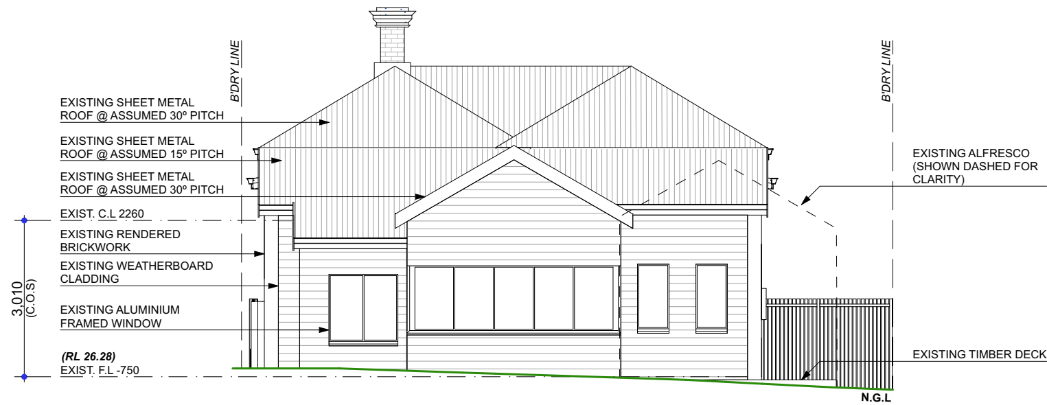
E03 A02 EXISTING ELEVATION 03 - EAST 1:100
