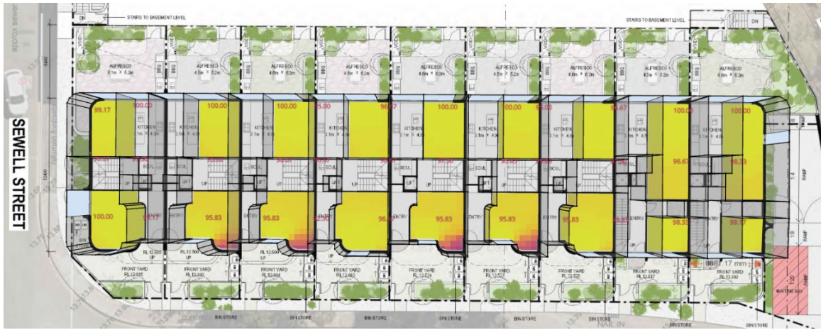
Figure 5: Daylighting for Ground Floor
