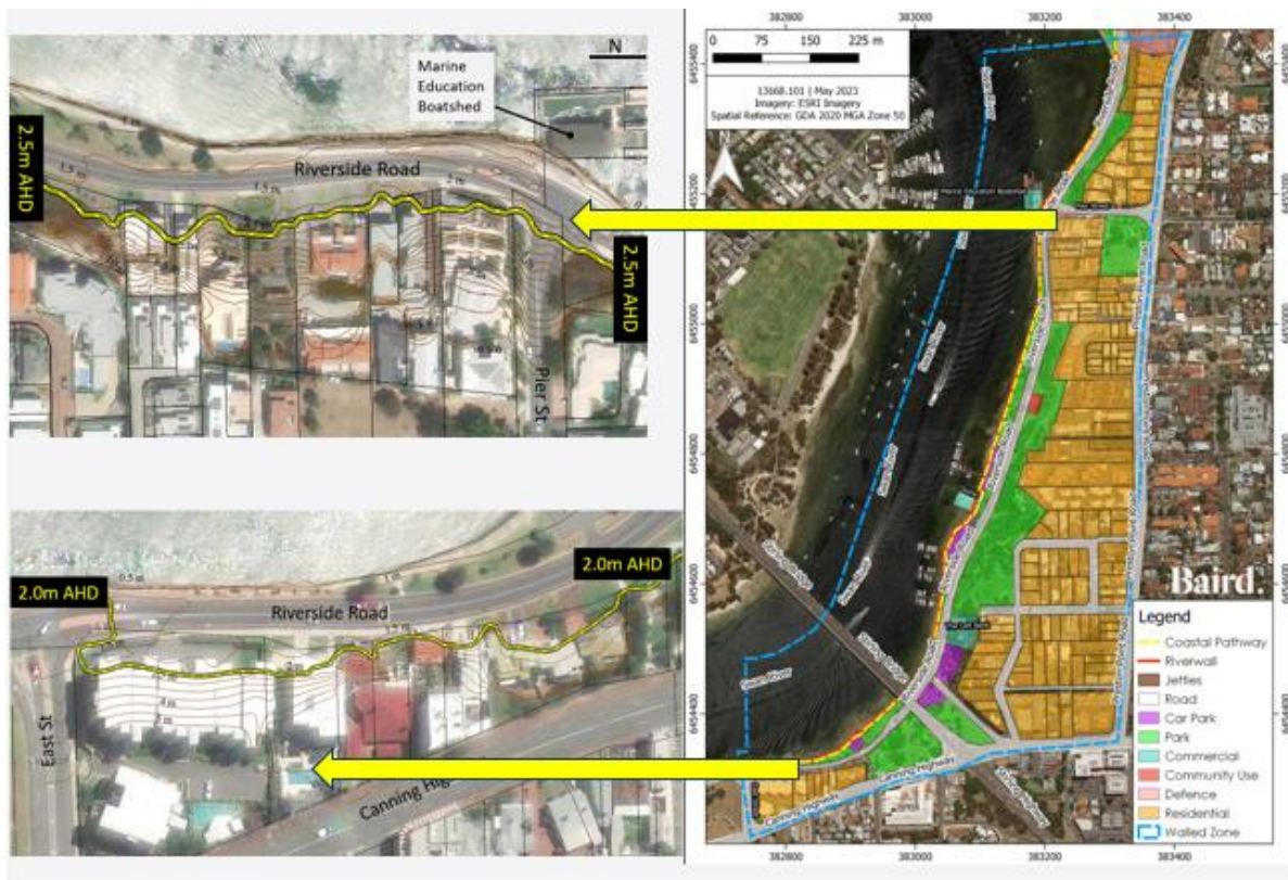
Figure 15.1: Inundation risk to existing properties on Riverside Road near Pier St and East St
