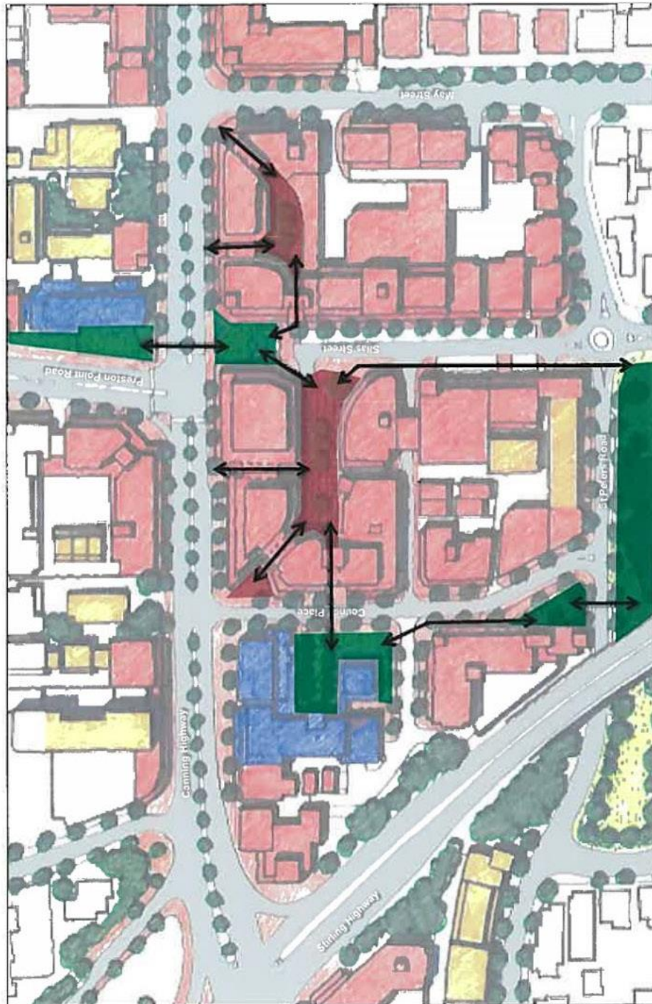
LEGEND Public space Urban space (privately owned but publically accessible) Plan 4: Internal pedestrian connections and public/urban spaces
