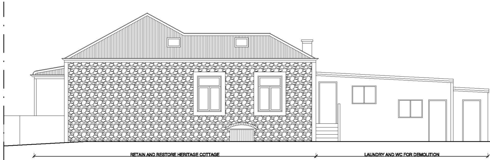
Existing Side Elevation (East)
