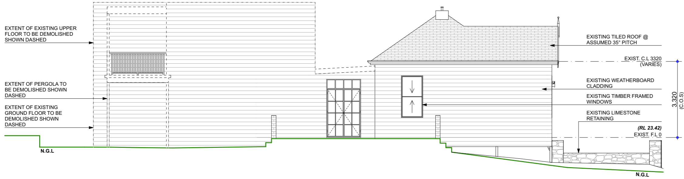
E02 A02 EXISTING ELEVATION 02 - NORTH 1:100
