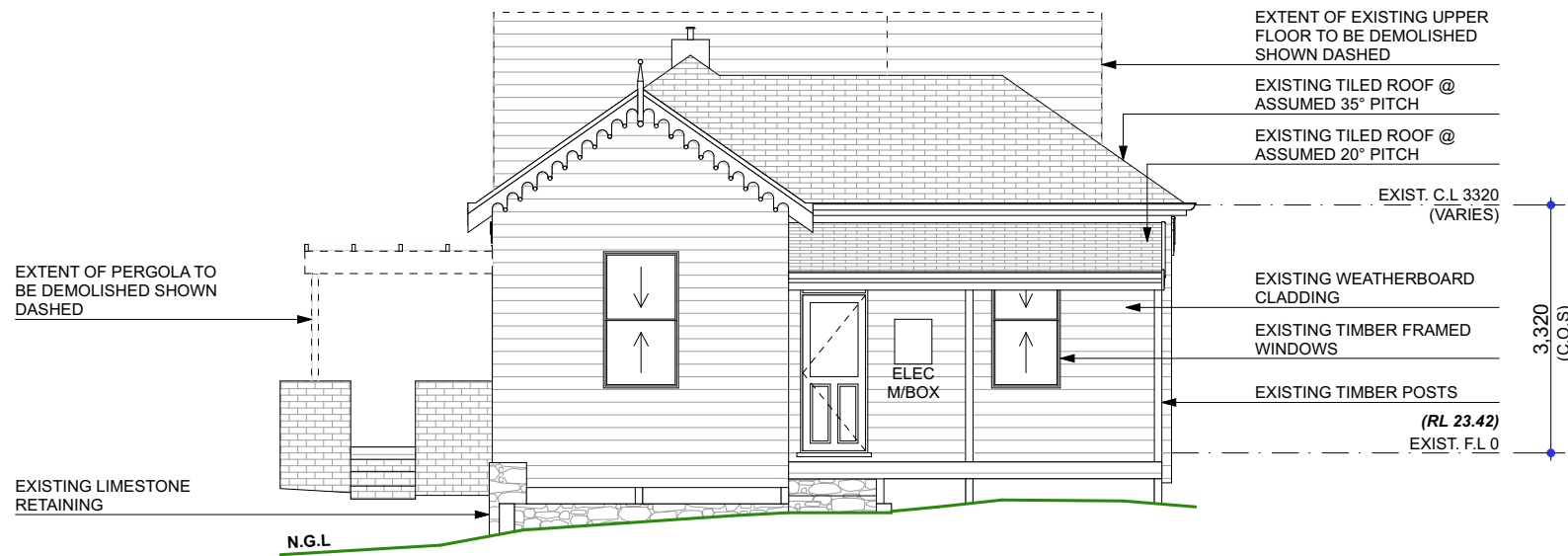
E01 A02 EXISTING ELEVATION 01 - WEST 1:100
