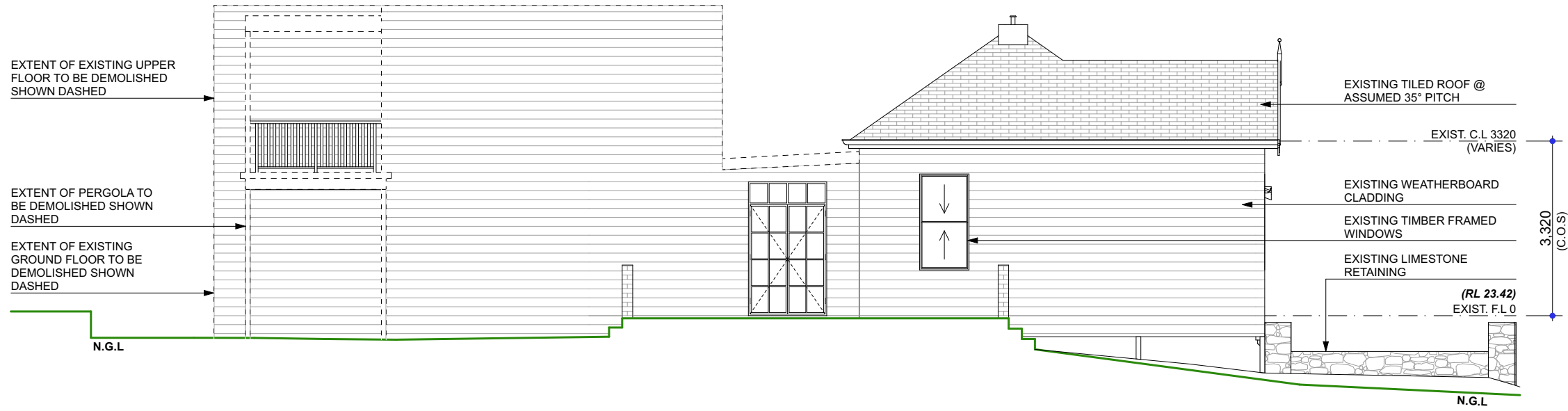
E02 A02 EXISTING ELEVATION 02 - NORTH 1:100
