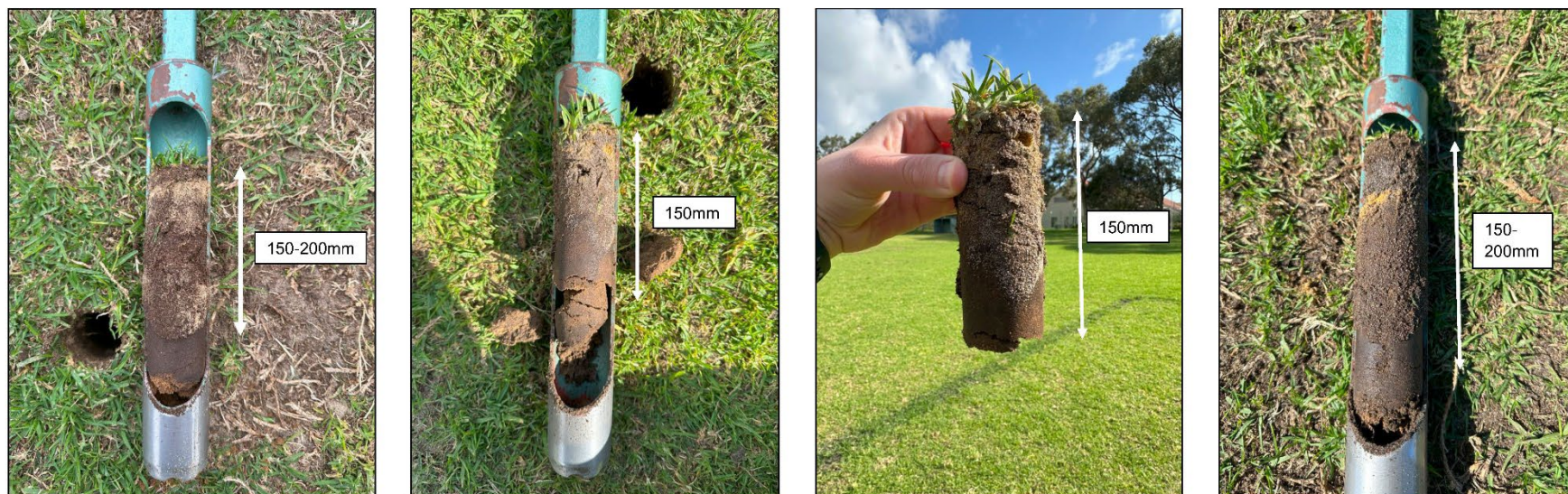
Images: 150mm – 250mm depth hard pan developing beneath the surface at each reserve.
