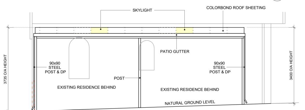
ALL CONC FOOTINGS & STRUCTURAL **ELEMENTS TO ENG DESIGN & SPECIFICATIONS**  PROPOSED STEEL FRAMED FLAT PATIO
