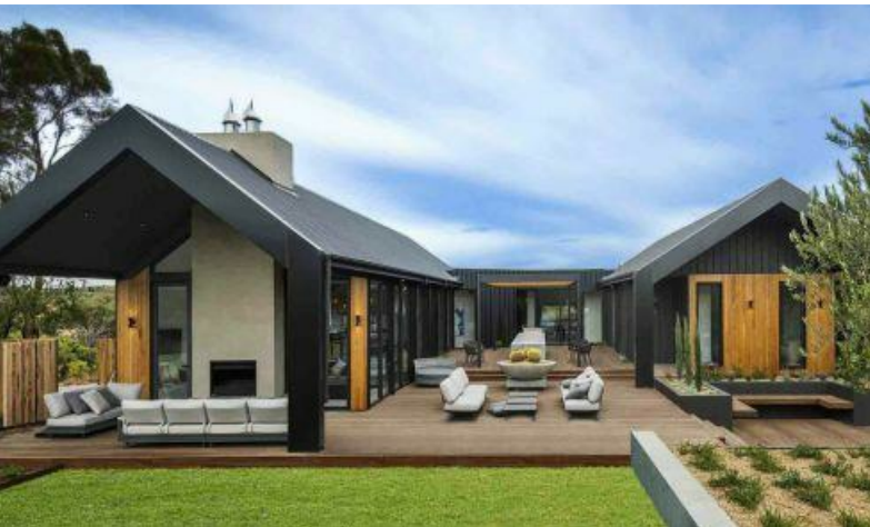
COLORBOND METALDECK ROOF AND FLASHINGS: MONUMENT COLOUR MATT FINISH POWDERCOAT ALUMINIUM WINDOW FRAME SAME COLOUR
