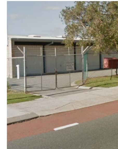
Image 14. Image shows grey footpath prioritised over crossover on Preston Point Road, East Fremantle. Source: google.com/maps, street view. Accessed 2019.
