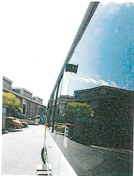
# Side Doors are hand crafted to be made flush with standard body shape, this allows for better resale in the future and also aerodynamics of vehicle .
