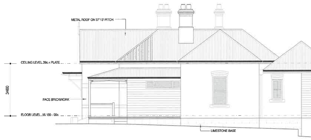
EXISTING HOUSE NORTH ELEVATION scale 1:00
